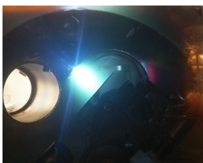
Fig. 1 Ho 2 O 3 plume formation via ablation using a KrF excimer laser pulse for thin film deposition.
